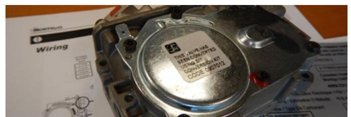
Figure 13.k Conversion label on valve
