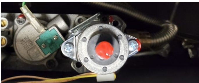
Figure 13.eee LP pressure regulator on a Full Load
